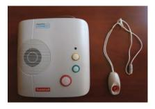
The lifeline unit is connected to sensors. The sensors are put around your home or can be worn round your neck as a pendant.
